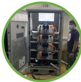
30KW/45KWh 鋰鐵電芯 (LFP)
